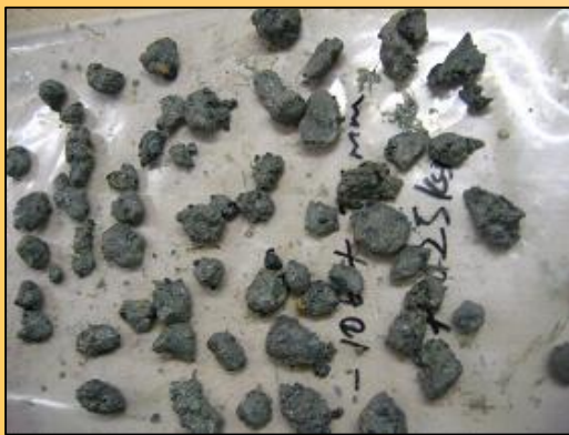
Kimberlite flake after deagglomeration in a scrubber
