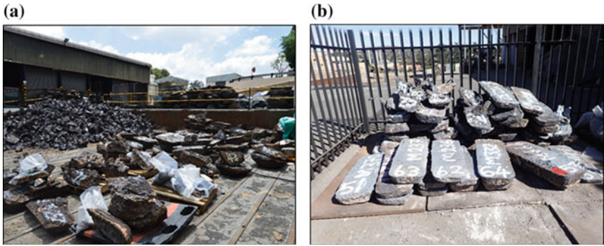
Fig. 7 Typical examples of a slag and alloy being manually separated in the slag waste area and b alloy being stored in the high-value shed
