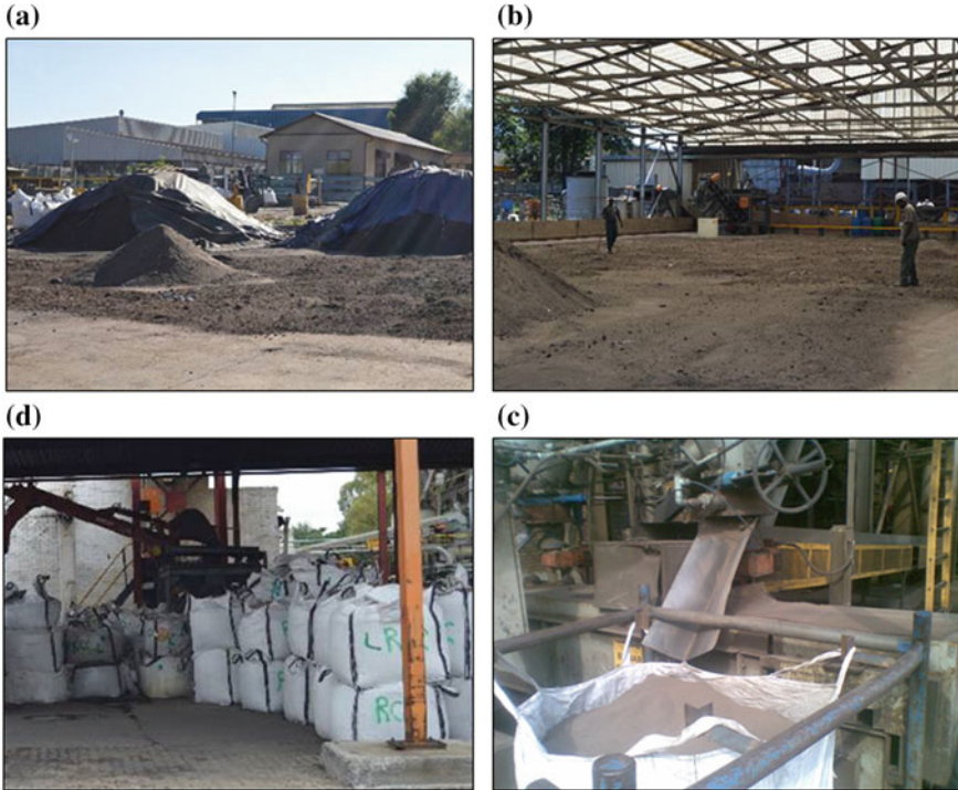
Fig. 2 Examples of raw material handling in preparation for a campaign: a raw materials stored in bulk under tarpaulins to minimise contamination, b raw materials being air-dried in a covered area, c dried raw material being bagged in bulk bags, and d bulk bags clearly marked and stored in covered area
